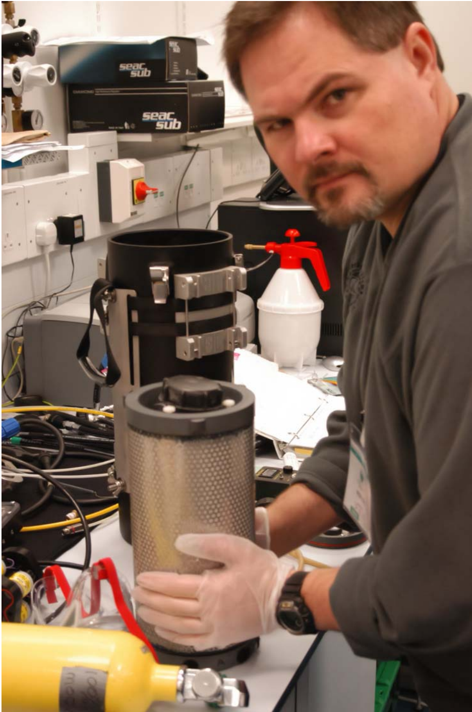
Photo 7 - Cis Lunar Scrubber Packing - Fits MEG
