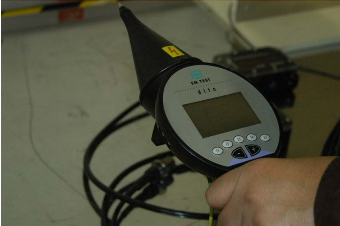
Photo 6 - The ESD tester - top static test discharge is 15,000 volts
